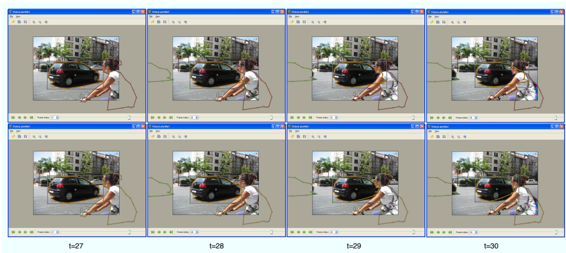
Figure 2.5. Occlusion reasoning is crucial for the correct tracking. Top row: the depth of the person is specified to be less than that of the car. The tracking was correct even though the car becomes occluded. Bottom row: the depth of the person is specified to be greater than that of the car. The tracking becomes wrong at the occlusion because the appearance of the person was mistakenly used for the appearance of the feature points of the car.
