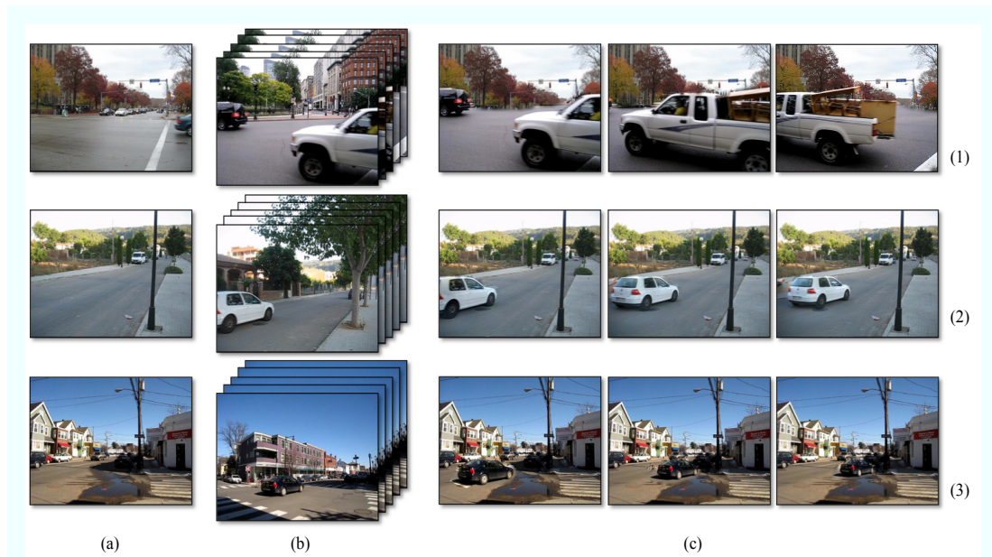
Figure 4.18. Motion synthesis via object transfer. Query images (a), the top video match (b), and representative frames from the synthesized sequence (c) obtained by transferring the moving objects from the video to the still query image.
